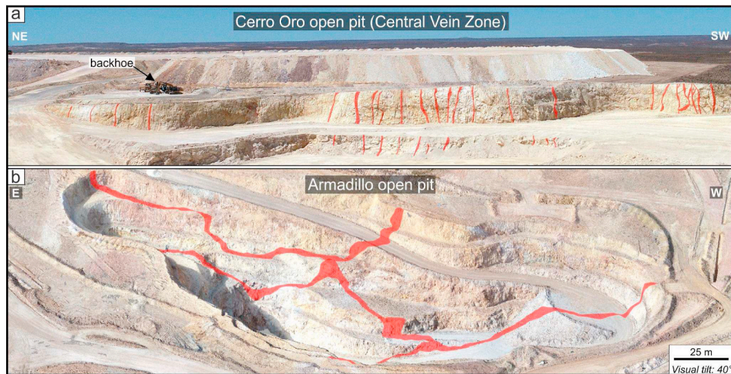
Fig. 4. Photographs of the open pits (a) Cerro Oro (CVZ) and (b) Armadillo, showing the structure of the vein/vein system.
